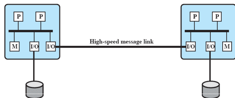
(a) Standby server with no shared disk
